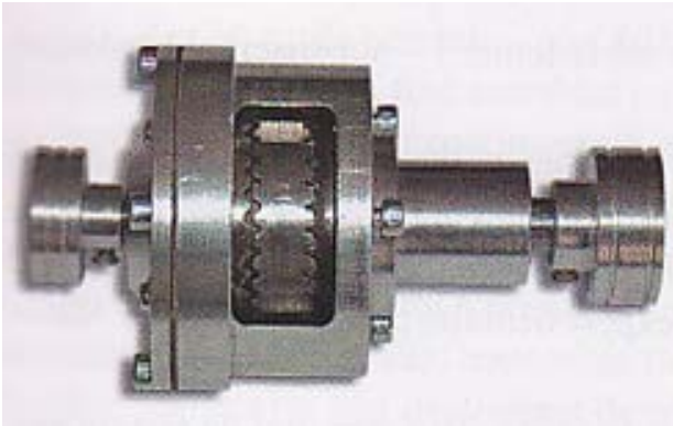
Figure 1. Planetary precesional kinematical gear box: a) Satellite wheel made of plastic material type Hostaform C2091 b) Satellite wheel made of powders material type Жр7.
